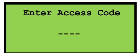
A Level 1 untrained user can view the current system state including any faults, alarms, disablements and tests. Level 1 users cannot access the Main Menu. See [3.1 – Quick Menu](#).
